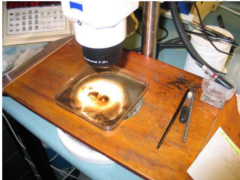
Fig. 4: Gridded Greiner tray used for sifting net tows.
