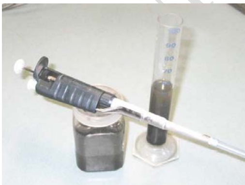
Fig. 6a: Gilson autopipette used to extract 1 ml from agitated trap sample
