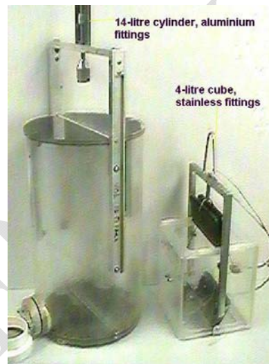
Fig. 3b: Perspex Haney plankton traps
